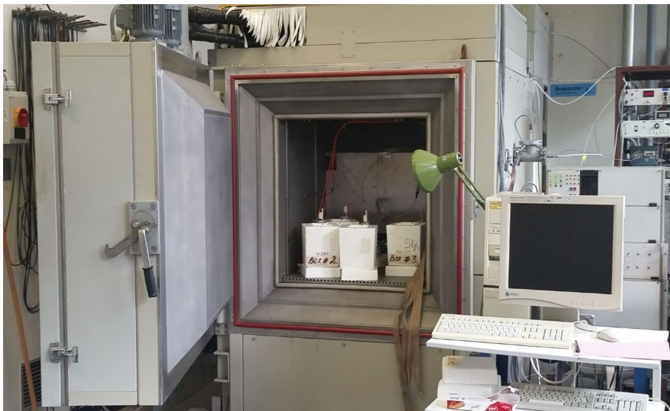
Figure 1. Environmental chamber at the Forschungszentrum Jülich with four ozonesondes positioned for a simulation run.
