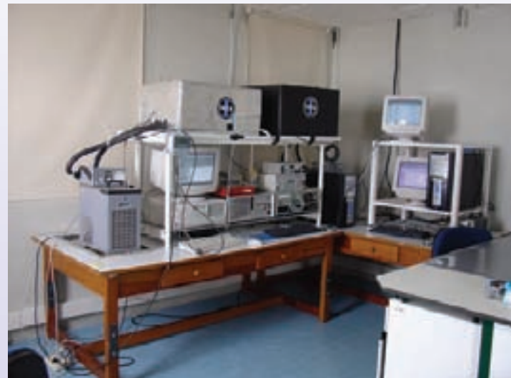
Photo 4. INTA PDA UV/Vis spectrometers are hosted in a laboratory located on the top floor of Izaña tower. Sunlight from the optical devices located on the terrace reach the instruments by means of a quartz fiber-bundle. Spectrometers are thermally regulated to minimize spectral shift and stretch.
